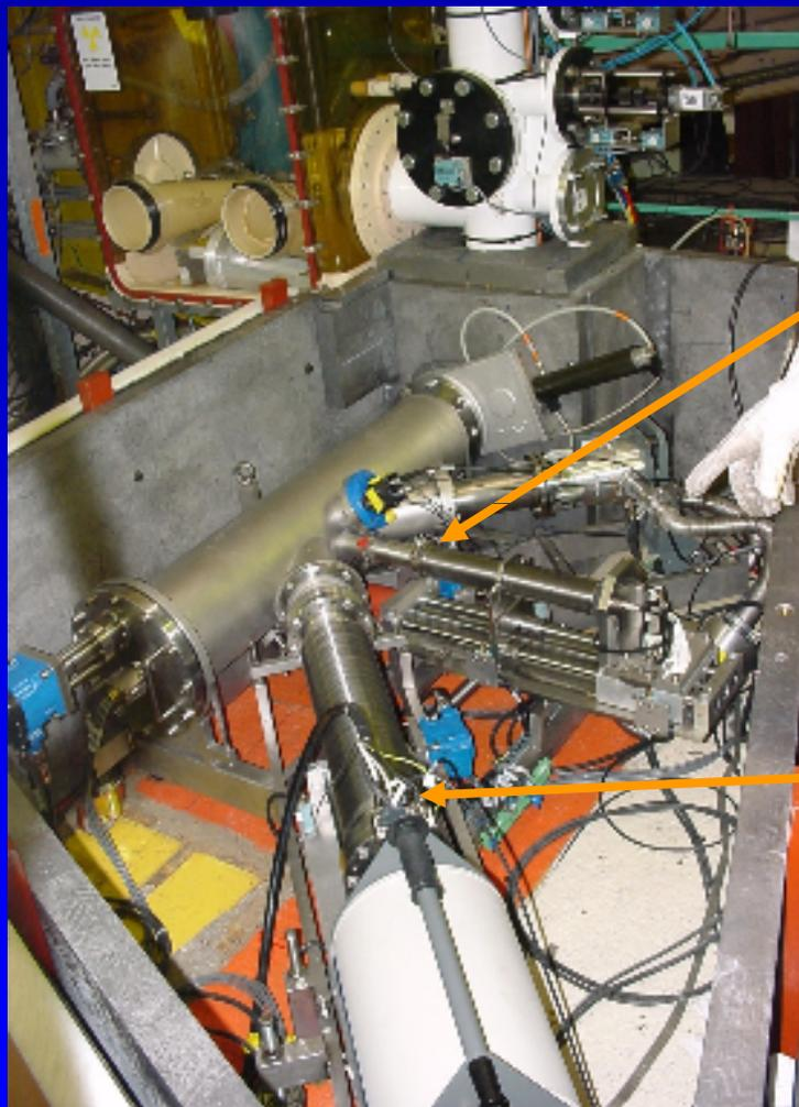
**PIPS detector (100  $\mu\text{m}$ )**
