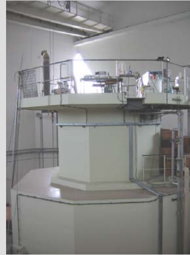
TRIGA Mark II at Jozef Stefan Institute, Ljubljana, Slovenia (max. power \approx 250 kW)
