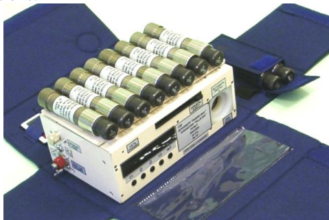
Fig. 8: The Pille TL dosimeter system in its transporting case (reader and ten dosimeters).
