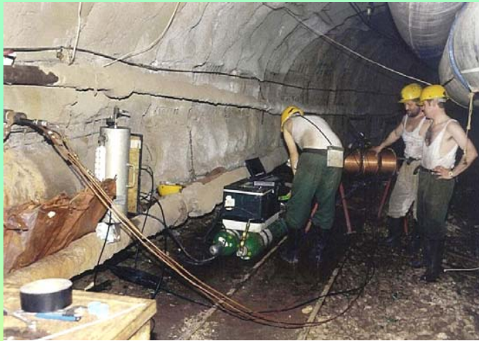
Implementation of a hydraulical test at the borehole Gamma-2 (performed by Golder)
